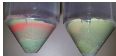
Figure 4. Visual comparison of as-synthesized CuCrO 2 samples; left: Mg-doped according P6; right: undoped according P5; Cu 2 O by-products visible as brick red precipitate
