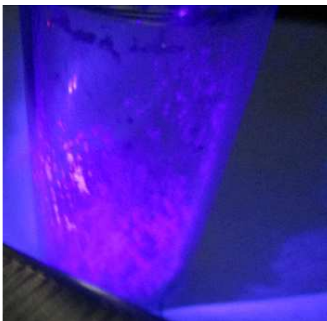
Fig. 5. Photo of PL from reduced Si nanoparticles.
