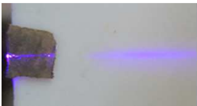
Fig. 6. Photo of PL from sintered Si nano-polycrystalline. Violet light for excitation was injected from the left side edge of the sintered Si nano-polycrystalline.
